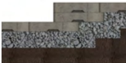
Install Base Course
